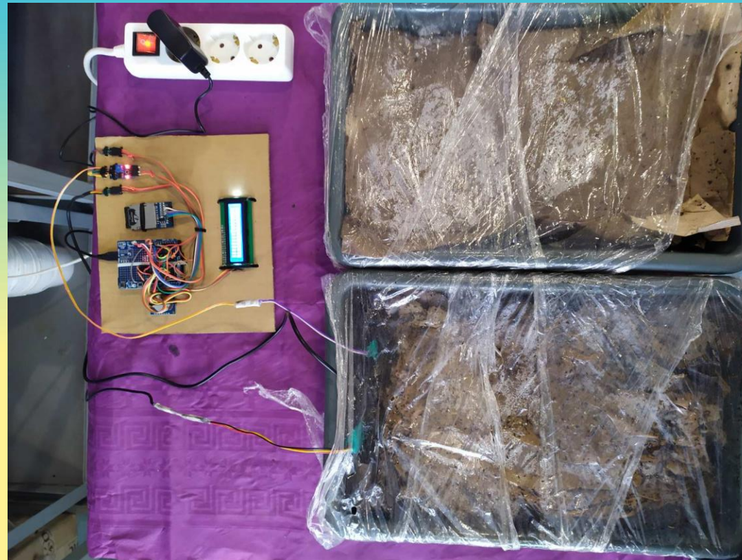
A pilot automated system for controlling soil moisture
